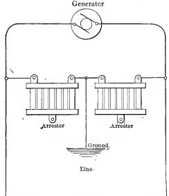
FIG. 108. Lightning arrestors connected to line and ground.
